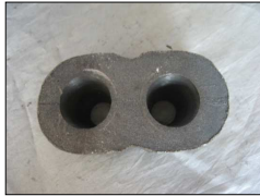
ANCHORAGE BLOCK 2CS13
